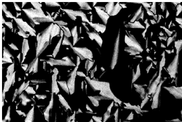
Figure 3. Defect texture of the columnar mesophase of N -palmitoyl cerebroside ( \times 100 ).
